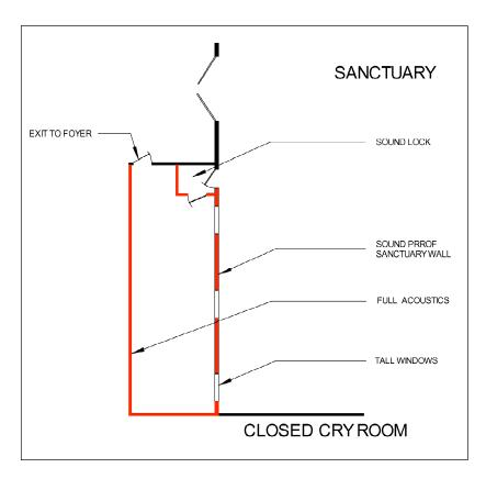
The soundproofing materials for the walls and ceiling should be capable of blocking the vibrations caused from the cries of children. A wall system that both isolates and dampens is typically the most effective.
